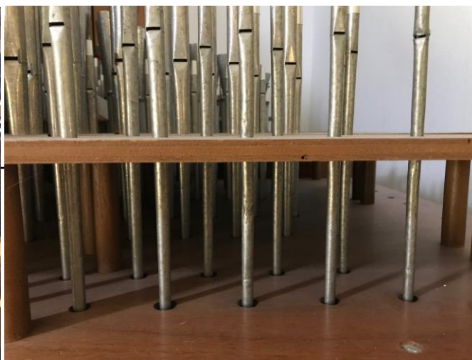
Pipes in the toe and rack boards.
